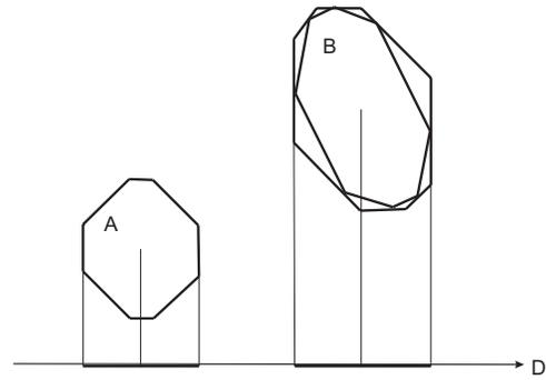
Figure 2: Approximation method using all  $k$ -DOP directions.
